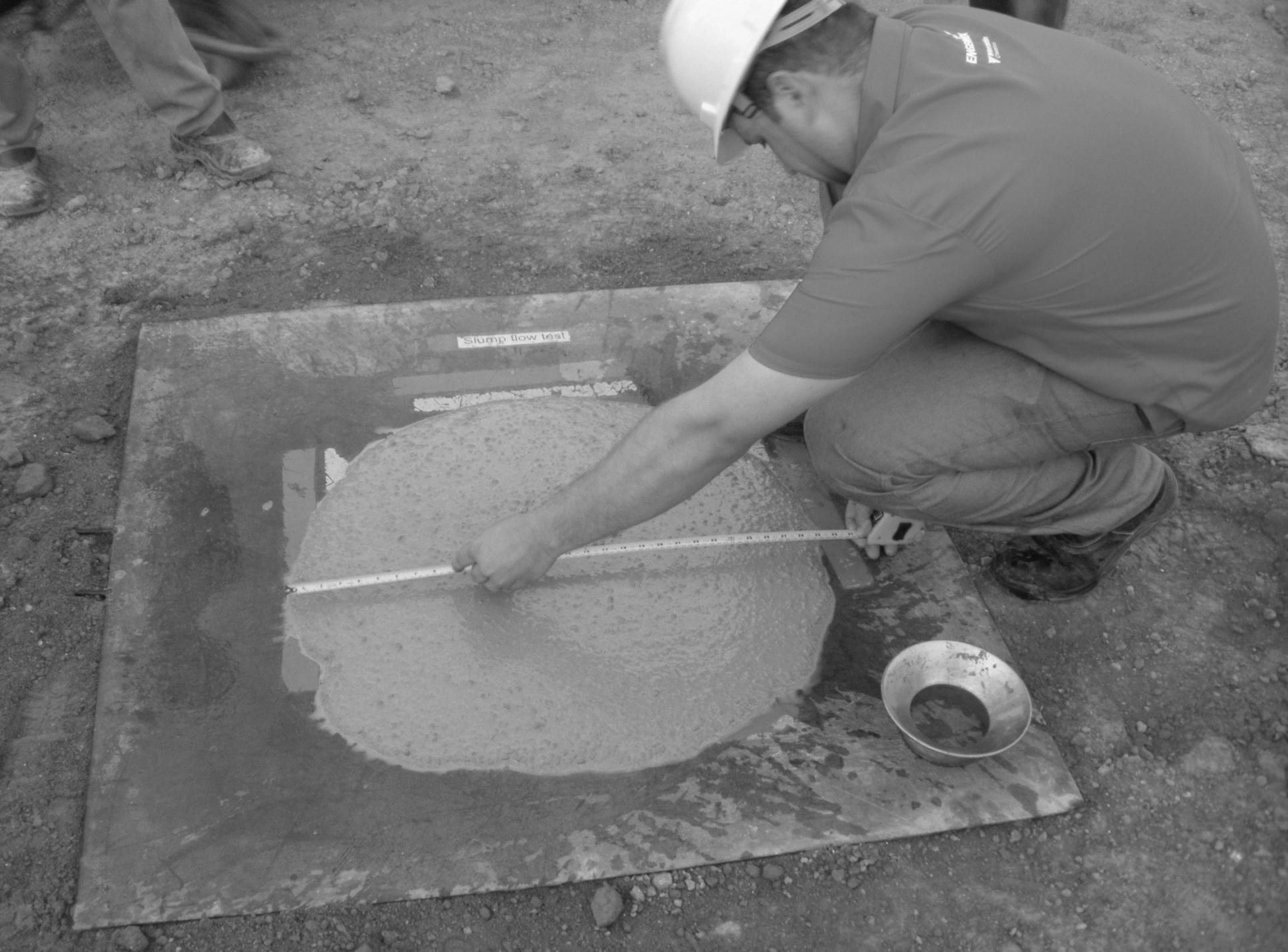
Slump flow test
